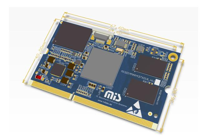
For a better mechanical stability the MIS-DIMM-AM437X can be fasten to the carrier board using the mechanical hole in the upper right corner.
