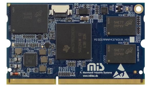
Texas Instruments Sitara AM437x based System-on-Module
